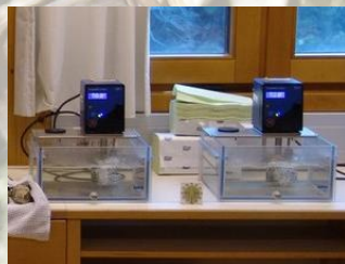
Fig. 4: Device setup for chlorophyll fluorescence measurements (Fv/Fm).
